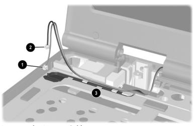
Removing the Antenna Cables
